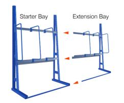
**2.** Connect the 2 side frames by attaching the 2 front beams and a back beam. Insert safety pins on both ends of all beams to secure in place. Attach the base rail using M6x16 nuts and bolts.
