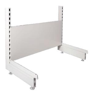
Insert base legs into uprights to make L shape for wall shelving or T shape for gondola shelving. To insert the base legs, locate the two upper lugs into the upright and rotate downwards to locate the lower lug, use a rubber mallet to tap the base leg into position
