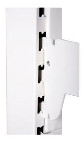
The brackets should be positioned in the H slot of the upright and should be located in the inside slot (the back panel and bracket for the next shelving bay will use the other slot). The 3 hook brackets can be horizontal or tilted upwards or downwards as required.
