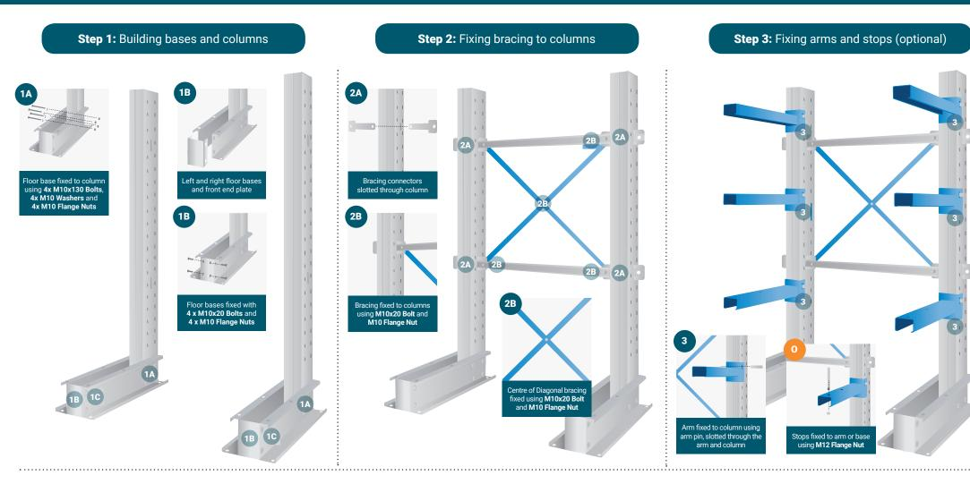
Position the column alongside the four fixing holes on the side of the right and left floor bases. To do this you will need to lift the column slightly off of the ground. Once aligned, fix the floor base to the column using **4 x M10x130 Bolts**, **4 x M10 Washers** and **4 x M10 Flange Nuts**.
